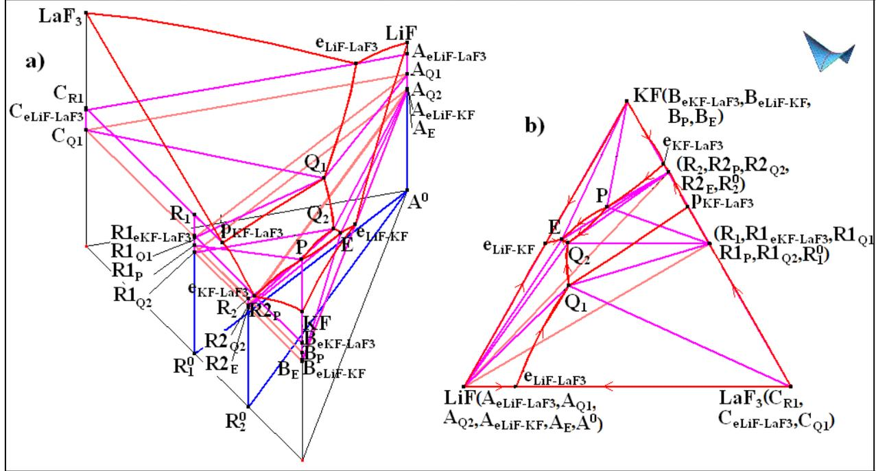
Fig. 1 Computer model of LiF-KF-LaF<sub>3</sub> system in prizm (a) and its XY projection (b)
