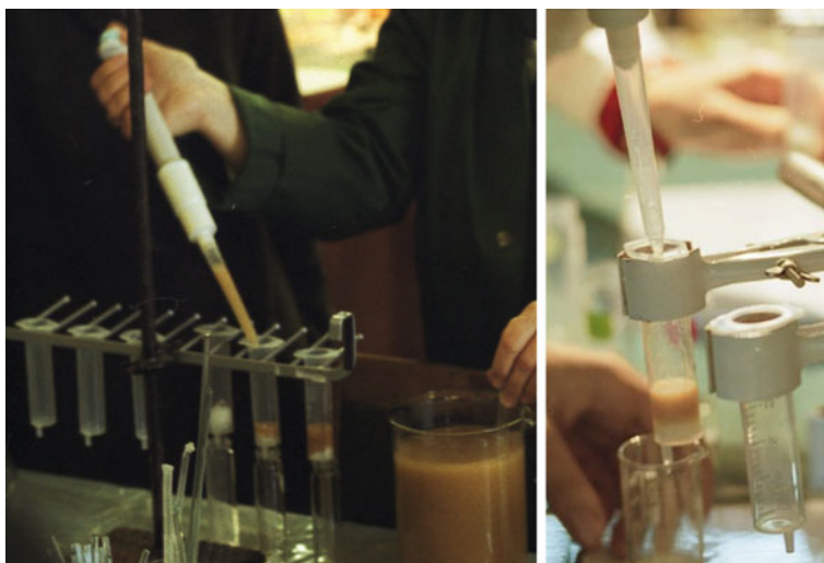
Fig. 4.3 Loading a suspension of an ion-exchange resin into columns with a dispenser and washing of the columns
