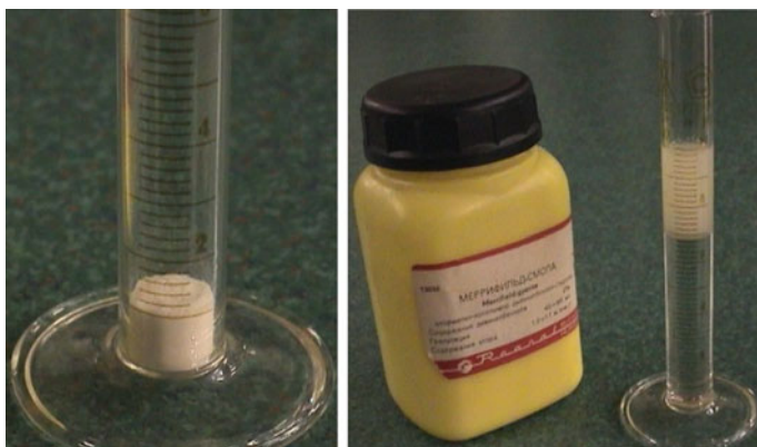
Fig. 1.1 Swelling of the Merrifield resin in \text{CH}_2\text{Cl}_2 (as seen, 1 ml of a granular material increases its volume 3 times)
