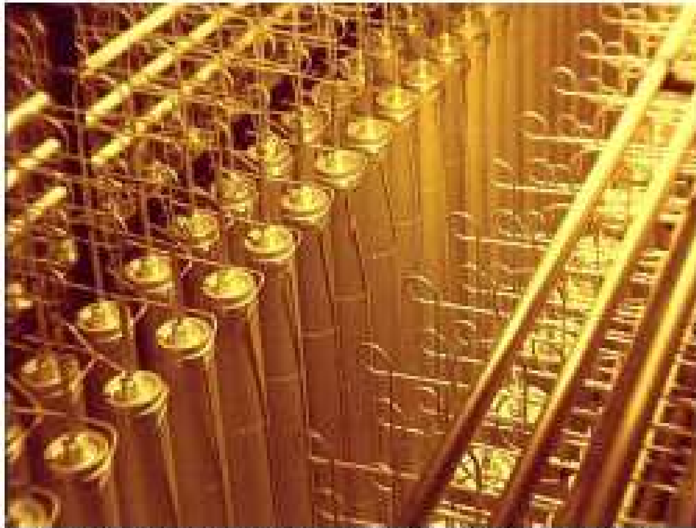
Figure 3: A section of a typical cascade of centrifuge stages in a European uranium enrichment plant. The separative power of each centrifuge increases with the speed of revolution as well as with the height of the centrifuge while in a cascade each centrifuge also builds on the enrichment achieved in the previous stages. photo taken from the Uranium Information Centre online at http://www.uic.com.au/uranium/centrifuge.html
