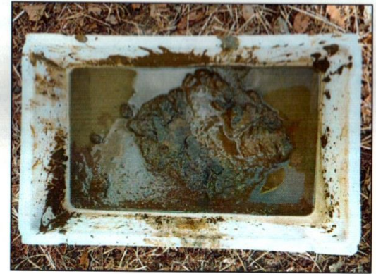
Sampling of bottom deposits (Smith-McIntyre Bottom sampler)
