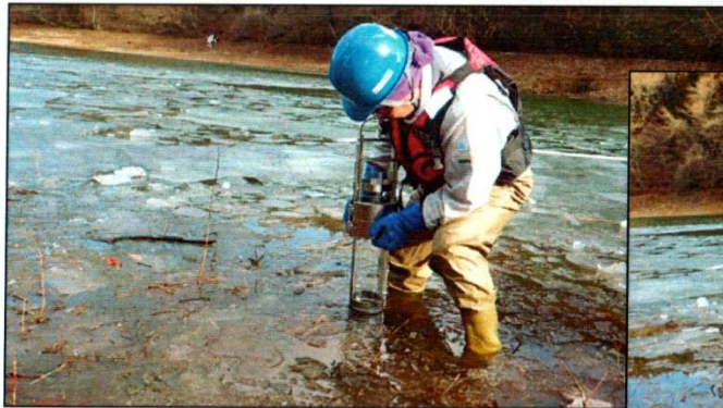
Core logging (undisturbed sampling)
