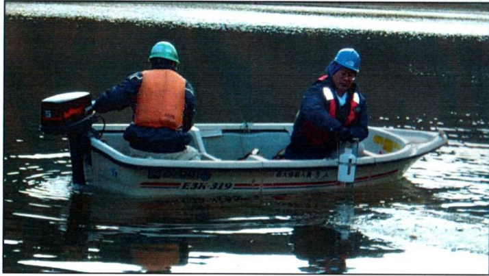
Water sampling (Heyroth sampling bottle)
