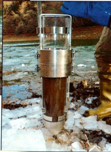
Core logging (undisturbed sampling)
