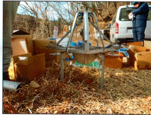
Sampling of bottom deposits (Smith-McIntyre Bottom sampler)
