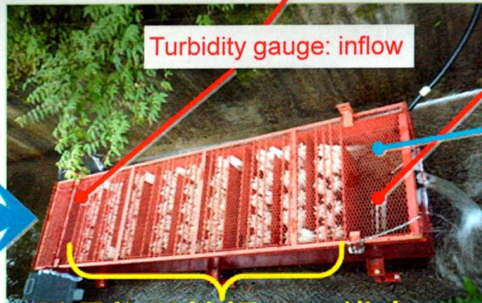
Traps of suspended solid in the river water by non-woven fabric
