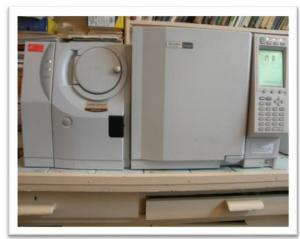
GC-2010 chromatograph and GCMS-QP2010S mass spectrometer
