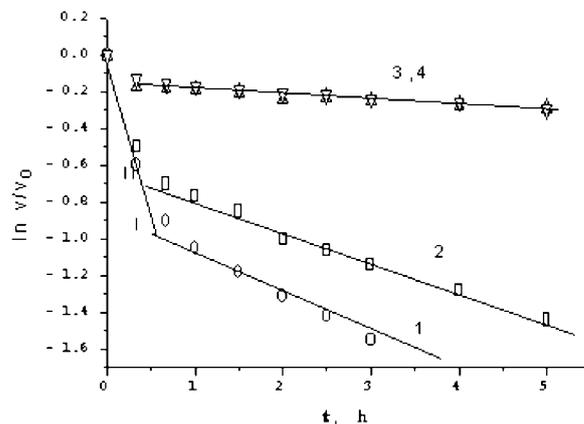
Fig. 2. Kinetic of thermoinactivation of  $\beta$ -galactosidase at pH 7.5 and 48°C and various concentrations of enzyme: (1, 3) 36.55 mg/l and (2, 4) 7.3 mg/l; (1, 2) in absence of  $\text{Mg}^{2+}$  ions and (3, 4) in the presence 0.01 M of  $\text{Mg}^{2+}$ .
